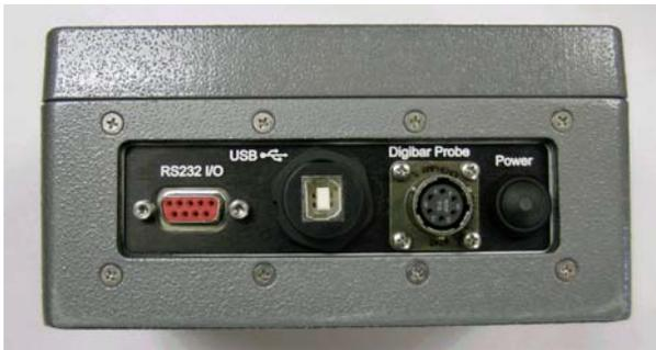
The junction box supplies power to the Digibar V probe and converts the RS232 data from the probe to USB so that it can interface to the pc. The junction box can also supply RS232 data to the pc. The junction box is powered up with the USB connector. If the USB port is not used to interface with a pc a USB power supply can be used to power up the junction box.
