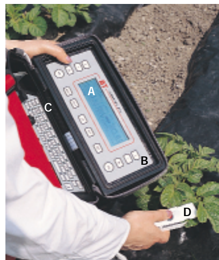
AP4 Porometer in use on potato crop growing through black polythene
