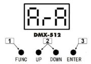
In the MODE OPTION setting, the stand alone laser show that you are going to choose is flashing. Press FUNC to change stand alone laser show, you will have 3 different stand alone preprogrammed laser show. Their DISPLAY and EFFECT are listed below:
