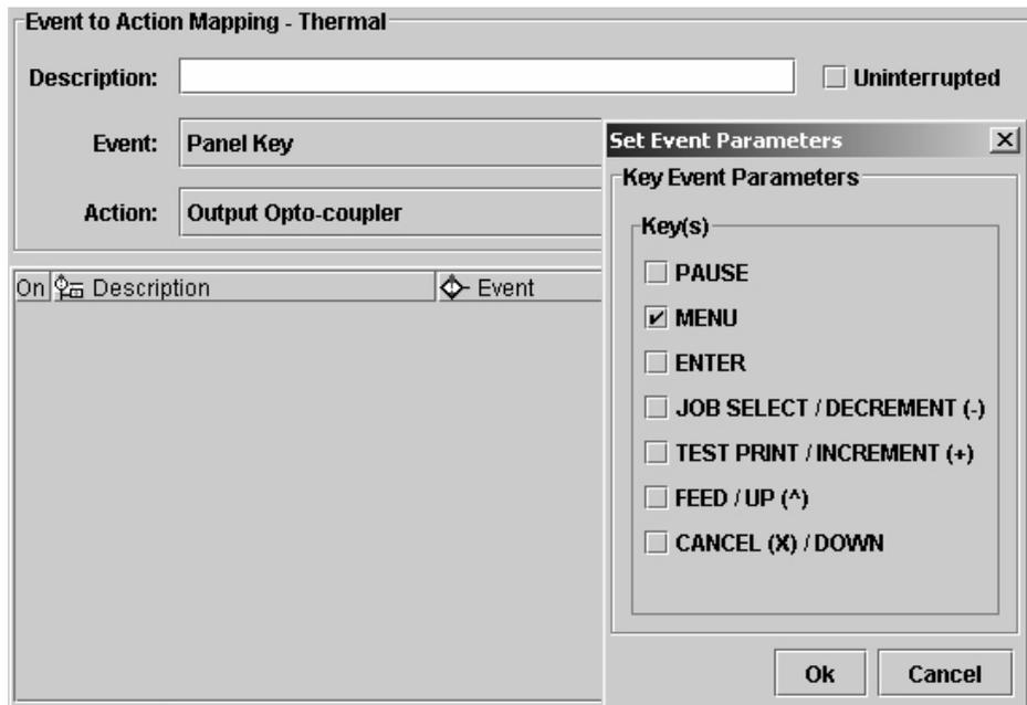
Figure 16. Setting Panel Key Event Parameters
