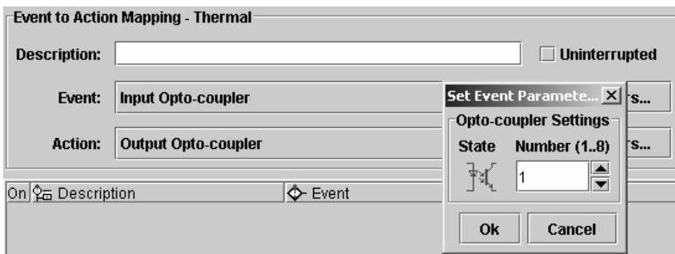
**Figure 14. Setting the Opto-coupler Number and State**
