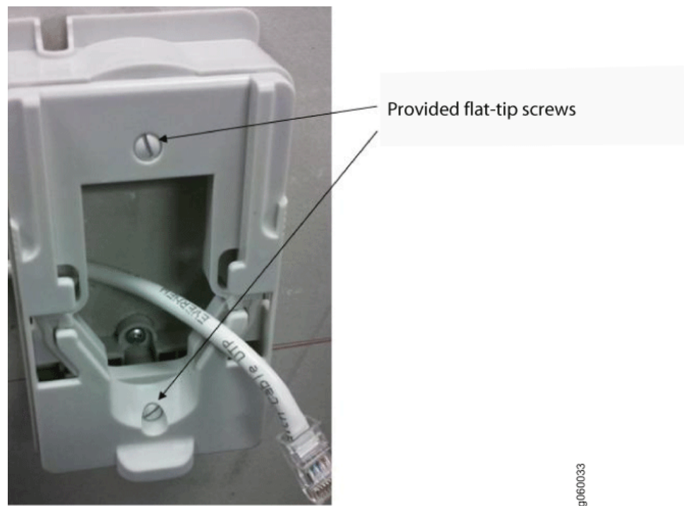
Figure 17: Faceplate Secured to the Wall-Mount Bracket
