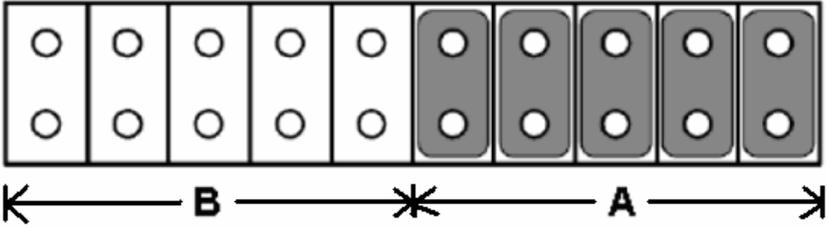
Jumper setting for RS-422/485 interface: (Default setting). (CN25/CN26)
