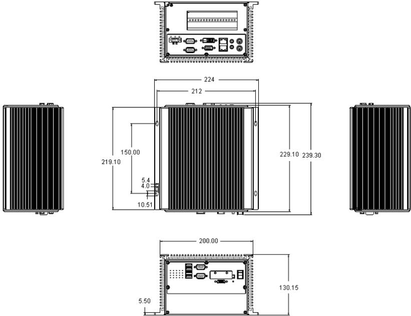
*Figure 1.1: Chassis Dimensions*
