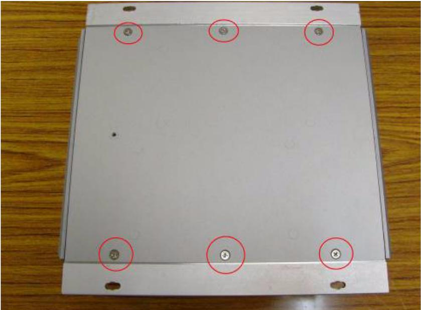
3. Move one screw to the center and it will make easy to remove the bottom cover.
