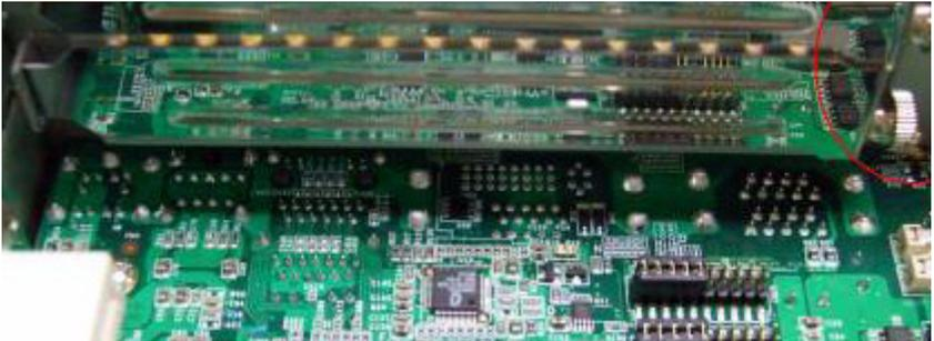
4. Plug-in PCI-bus card in a PCI-slot of UNO-3282.
