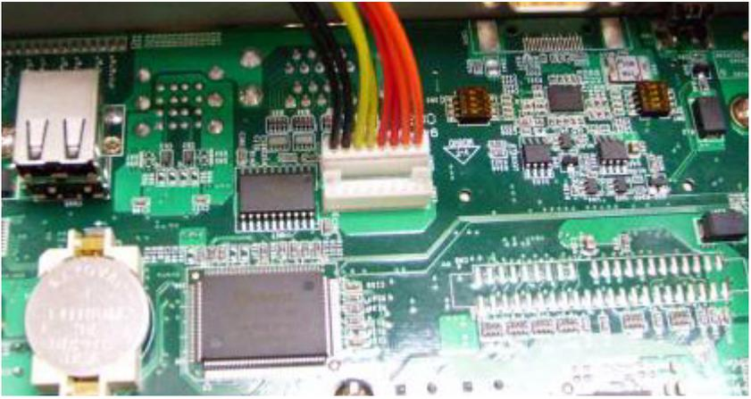
6. Connect the SATA cable with SATA connector (CN16 or CN18)
