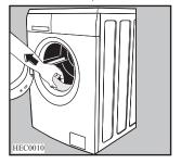
Open the porthole and remove the polystyrene block fitted on the door seal.
