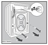
5. Open the porthole and remove the polystyrene block fitted with the adhesive tape on the door seal.
