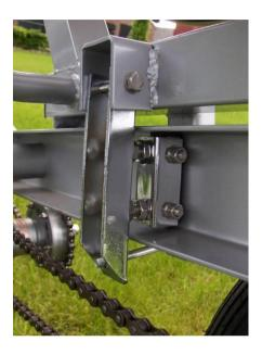
If the seat is clamped with high force to the frame, but it can still move sideways, the horizontal clamping only happens at the top or bottom of the clamp block. One can check with a feeler gauge whether the clamp block is in contact with the frame beam over the full height. If one side is not touching the frame beam, use the M8 nuts at that side to push the clamp block further to the frame beam.
