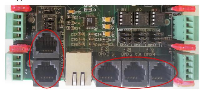
The 2 RJ45 jacks labeled J3 and J4 can be used as an E1.31 to DMX bridge, *or* as input/output from a standard LOR RS485 network depending on configuration.
