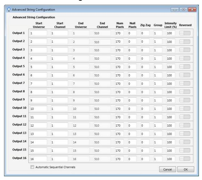
This allows for advanced configuration of the 16 pixel ports. Each port can be individually configured for its start universe, start channel, number of nodes (or pixels), null pixels, zig-zag and reversing. By using combinations of these options it can make setting up your pixel fixture more practical and simple, and often also results in shorter sequencing times.
