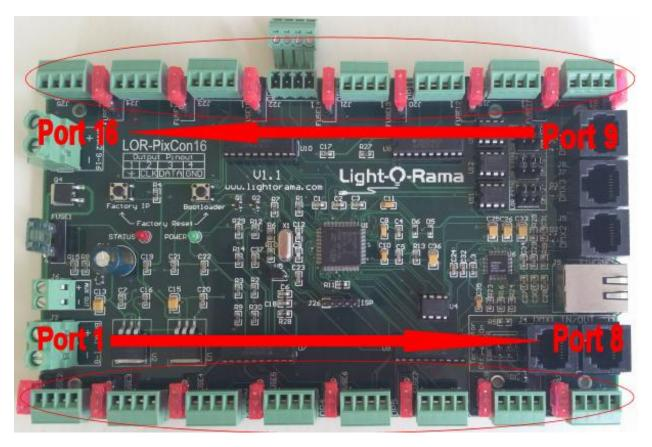
Connect up to 340 pixels to each port in E1.31/DMX mode, and up to 170 pixels to each port in Enhanced LOR Mode. The board can support several different pixel types, but all ports MUST have use same pixel driver/type. For example, you cannot mix WS2801 and WS2811 pixels on the same PixCon16.
