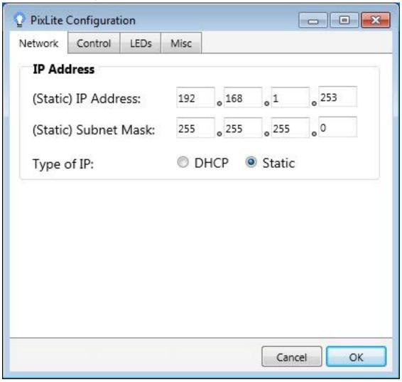
Here you can specify the static IP address and subnet mask that the controller will operate on as well as the type of IP connection. (Use DHCP to instantly see and configure the controller on any existing LAN.)
