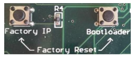
A factory reset should only be performed when absolutely necessary. The reset will erase all configuration and networking information which may be time-consuming to restore.
