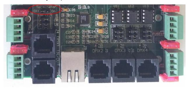
Should you experience data transmission problems when using the PixCon16 on an LOR network, you may want to move this jumper from OFF to ON. Most networks will not require this.
