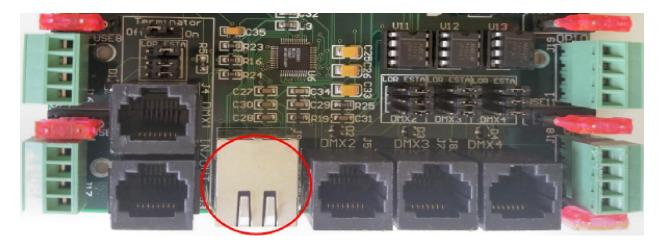
Use this port to connect the PixCon16 to your network or computer's network card. All configuration is done while the board is attached to a network via this connector.
