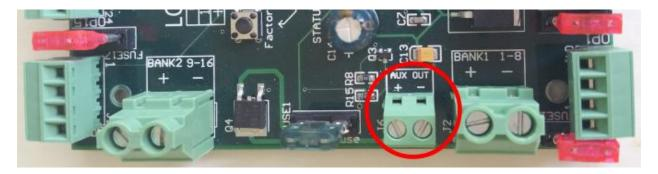
The Aux Out connector supplies power for an optional case fan. The fan's speed can be varied by temperature and is set by the Configuration program. Please note that the power for the fan is taken from Bank 1. You should select a fan that has the same voltage as Bank 1.
