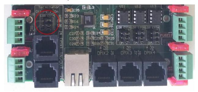
Whenever LOR equipment is in use on any of these RJ45 jacks, the jumpers must be moved from the ESTA side to the LOR side. LOR controllers, even in DMX mode, use a different pinout than other devices. Moving these jumpers sets the correct pins.
