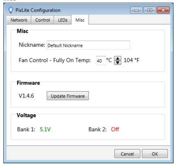
This allows the user to assign a custom nickname to the controller, perform a firmware update and also displays the current bank voltage of each of the two main power banks.
