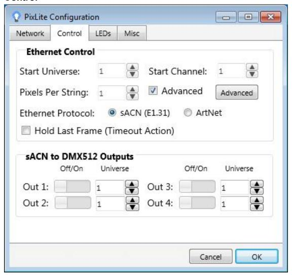
This window allows you to automatically setup a pixel fixture very quickly by simply specifying the start universe, start channel and the number of pixels in the fixture. The utility then automatically allocates the correct sequential universe addressing for all the pixels in the fixture for you. This is very useful if your fixture has the same number of pixels on each of the 16 outputs.
