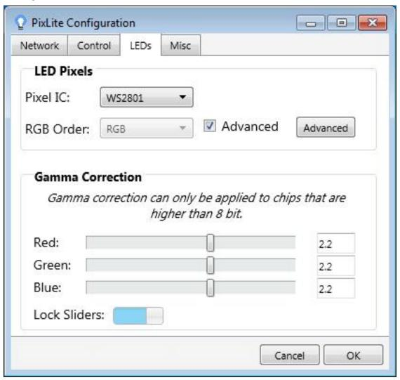
This allows you to select the type of pixel IC you wish to control as well as gamma correction (only applicable for strings that have greater than 8 bit data capacity). You **cannot** mix different pixel drivers (chips) on a single PixCon16 controller. For example you can't run the WS2811 protocol on ports 1-8 and SM16716 on ports 9-16. All 16 ports must be of the same type.
