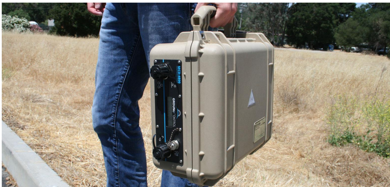
The MCD-4800 is watertight, and operates with the case lid closed.
