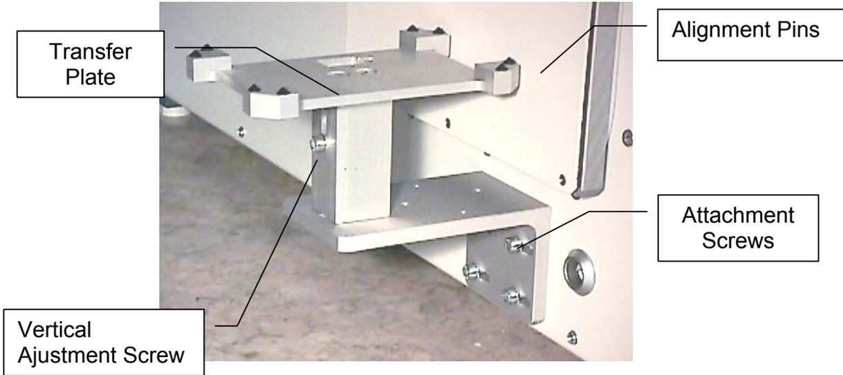
The transfer station can easily be adjusted. The transfer plate can be adjusted horizontally and vertically. Rotation of the transfer plate can also be adjusted.
