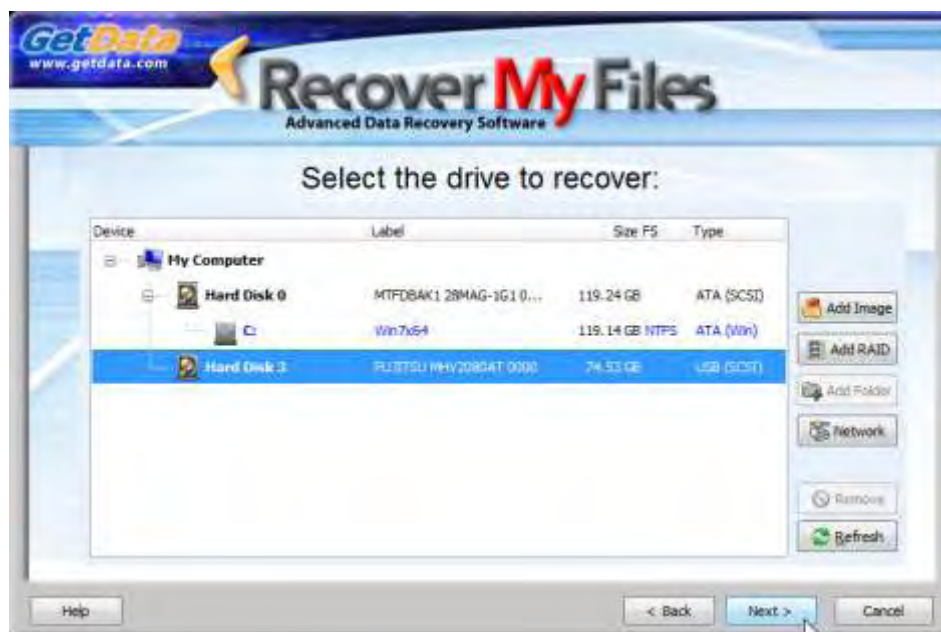
Figure 57, Drive selection screen, showing "Hard Drive 3" which has lost its drive letter
