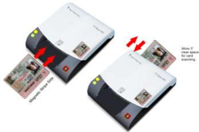
**Insert the identification card into the scanner**
