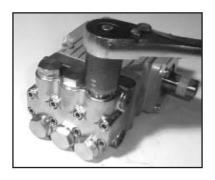
1. With a 22mm socket wrench, remove the (3) discharge valve plugs and (3) inlet valve plugs (32) Inspect the o-ring (33) for wear and replace if damaged.
