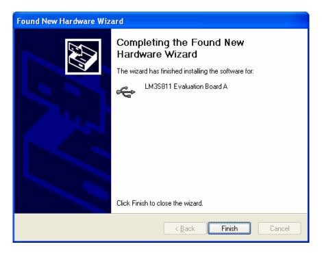
You have just installed the drivers for "LM3S811 Evaluation Board A." The USB device built into the EVB is a composite USB device. After you click Finish, a new Found New Hardware Wizard appears asking to install drivers for another device. This is for the "LM3S811 Evaluation Board B" part of the composite USB device. Follow the same instructions as above to install the drivers for this device.
