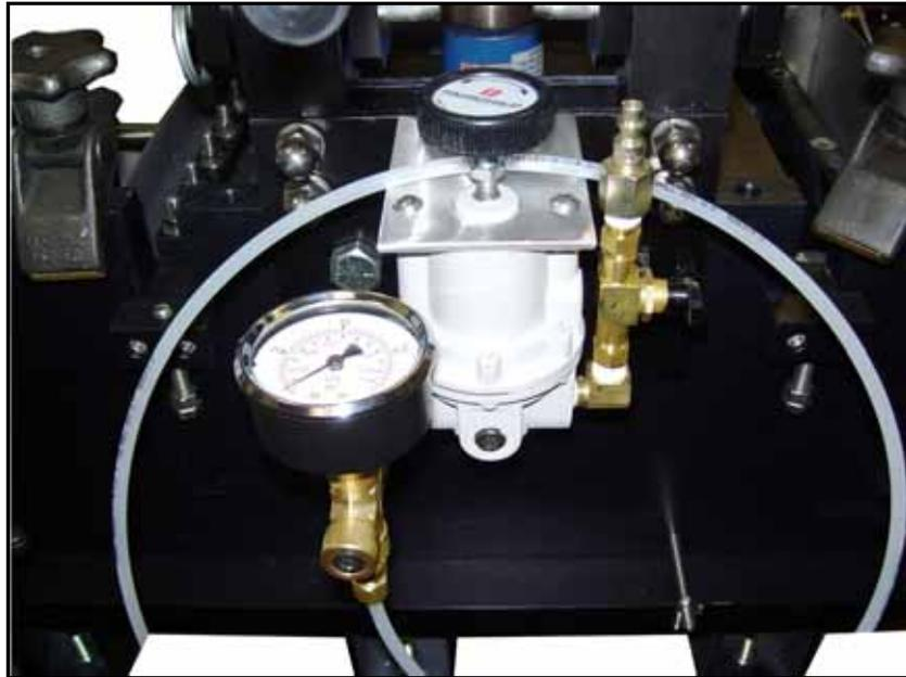
Regulator for controlling the normal load.
