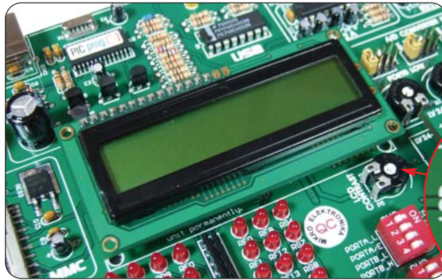
LCD 2x16 in 4-bit mode
