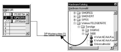
Next, using the same method as above, drag the modules from the hardware catalogue into the box for the field unit. Note that the 4-word module must be placed into cell 0 and the 6-word module into cell 1.
