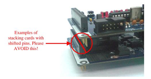
**Cautions:** Please ensure that all card pins are not shifted when stacking. IFC system will NOT function if the pins are shifted.
