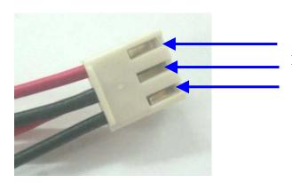
Ensure the iron pins are fully inserted to the connector
