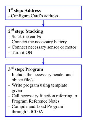
There are 2 basic setups in this chapter for IFC-OC04, the first one includes 3 cards, IFC-PC00, IFC-MB00 and IFC-OC04, and second one includes one extra card, which is IFC-CP04. Please refer to the following part of this chapter for setup details.
