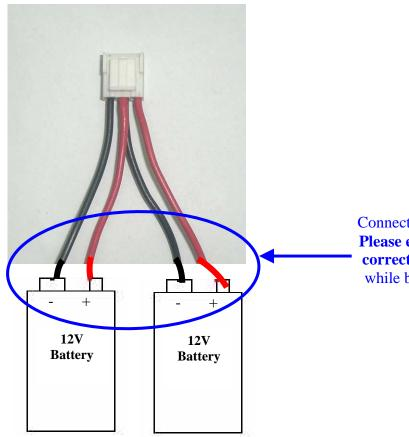
Connect the cable to batteries. **Please ensure the polarity is correct.** Red for positive (+) while black for negative (-).
