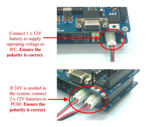
f. Connect the External power source for Output Card. Please refer hardware setup for connecting power to Output Card.
