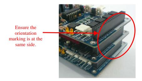
**Cautions:** Please ensure that every card is being stacked properly in correct orientation. Whole IFC system will be damaged if one of the cards is being stacked wrongly when it is powered up.
