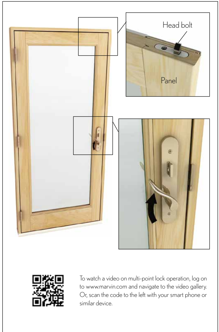
Figure 1 Lifting the handle upward will engage both the head bolt and foot bolt.
