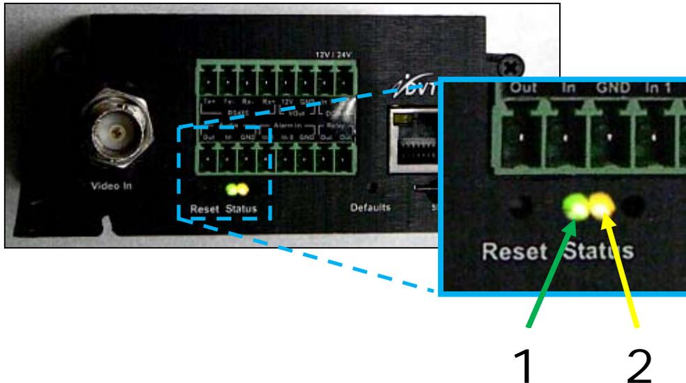
In addition to the status indicators, there are LED lights for the Ethernet 10/100 connector that operates when the unit is connected to the LAN:
