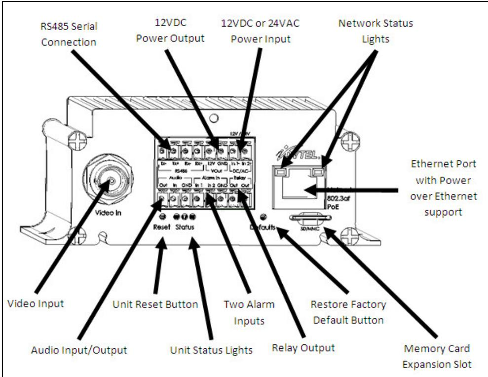
The following diagram shows a close-up view of the terminal block connection for the EA-201-0 encoder unit.
