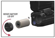
4. Remove Battery Lid using coin. Place provided battery positive (+) side toward trigger guard. Screw battery lid back into place. When changing the batteries, swab the threads of battery cap and the body with isopropyl alcohol or dry cotton swab.
