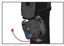
Attach Rail Master Pro at desired location on firearm rail and rotate into place, aligning insert with rail lug. Turn screws clockwise to secure clamps to rail.
