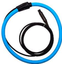
Flexible clamps F-2 (Rogowski coil) with a diameter of 25 cm (perimeter: 80 cm)
