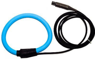
Flexible clamps F-3 (Rogowski coil) with a diameter of 13 cm (perimeter: 45 cm)
