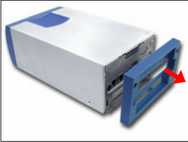
Fig. 2-6 Take off the plastic back panel
