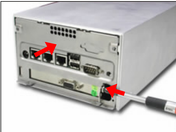
Fig. 2-40 Fix the PCI card to the back panel
