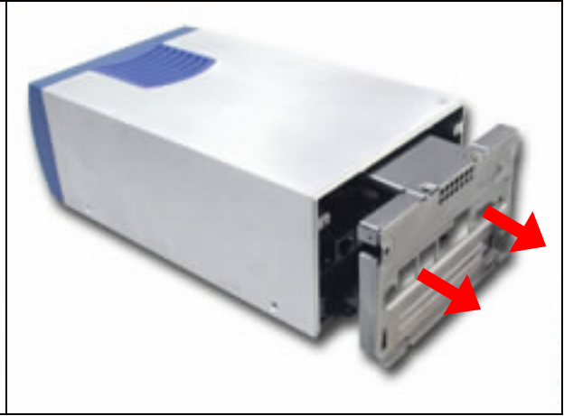
Fig. 2-7 Pull out the inner steel case
