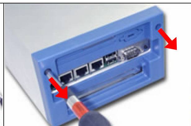
Fig. 2-4 Take off the screws on back panel
