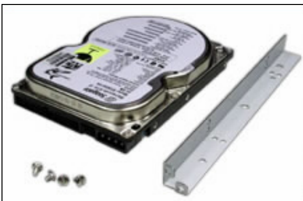
Fig. 2-26a A 3.5" HDD and the HDD bracket
