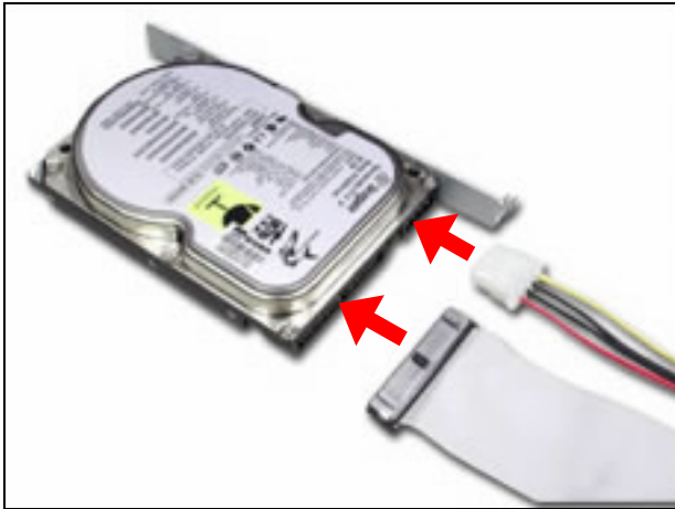
Fig. 2-27 Connect power and IDE cable to HDD
