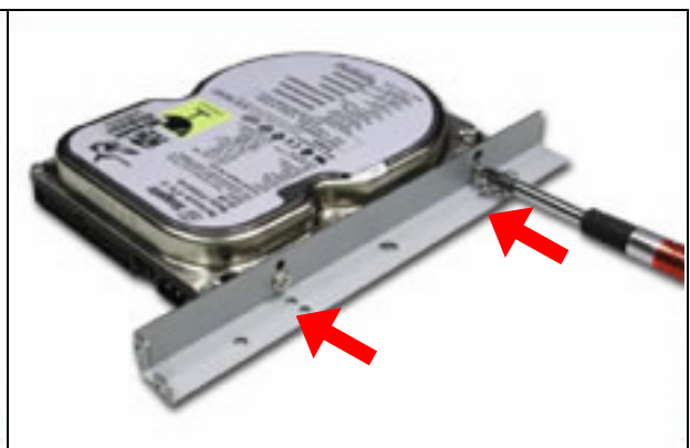
Fig. 2-26b Fix HDD to the bracket
