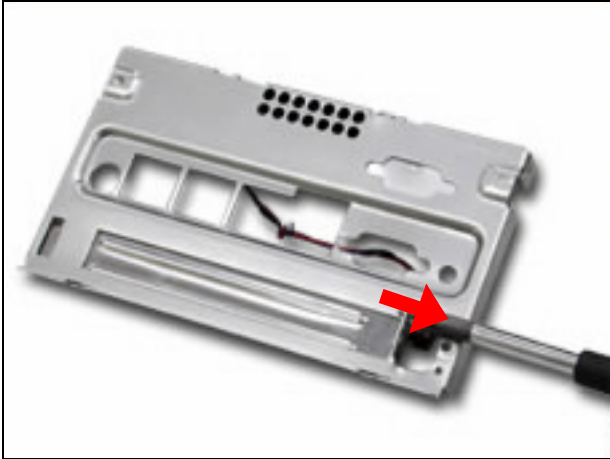
Fig. 2-38 Remove the original metal bracket
