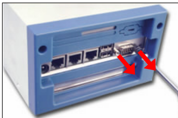
Fig. 2-3 Remove bolts from COM port
