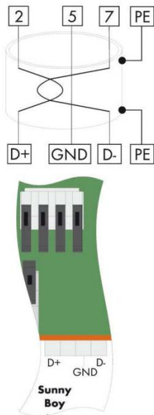
9. Shorten unnecessary conductors back to the cable sheath to prevent short circuits occurring.
