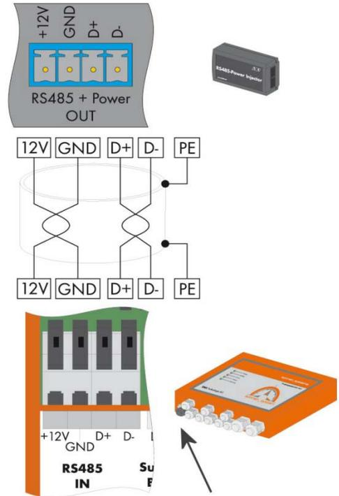
10. Connect the RS485 power injector to the SOLTRK as shown in the figure above. Refer to the table for details on the twisted pair cables.
