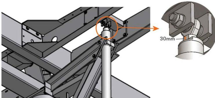
2. Press the UP (0°) key
