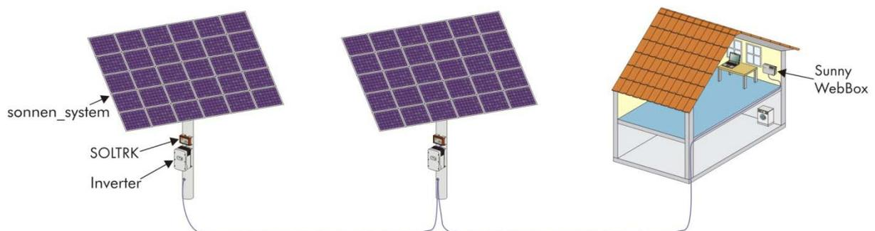
Up to 50 units (SOLTRK and inverters) can be managed by one Sunny WebBox. The travelling range of the tracking system can be restricted to prevent or reduce reciprocal shadowing of the sonnen\_system installations (track-back).
