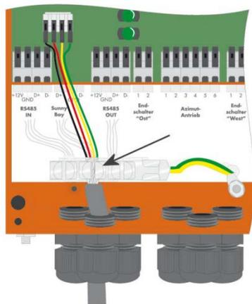
8. Connect the wires inside the SOLTRK to the “Sunny Boy” connection (see figure below).
