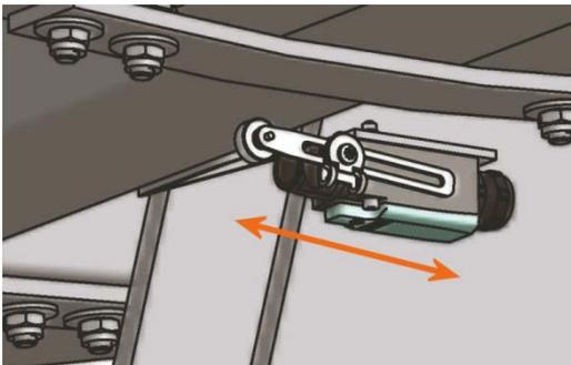
3. Push the twist lever under the central beam until the 0°-limit switch audibly switches over.
