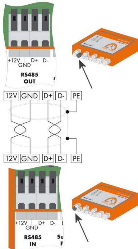
11. Connect the wires to the "RS485 IN" connection on the other SOLTRK as shown in the figure above. Use the conductor colours you noted earlier.
