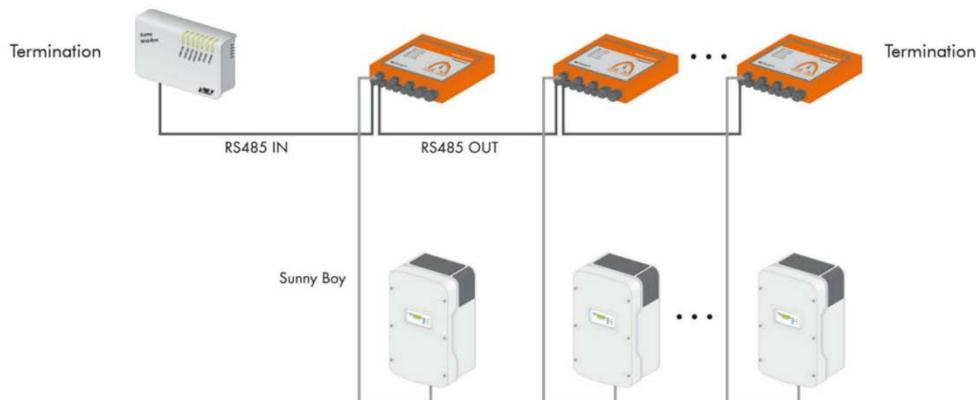
The following devices can be found at each of the two ends of the RS485 data bus and must be terminated accordingly:
