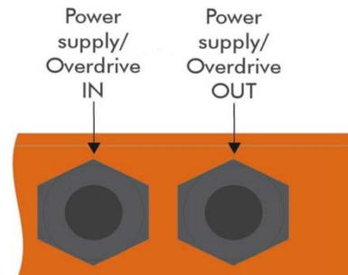
3. Connect the power supply and overdrive line inside the SOLTRK as shown in the figure below.
