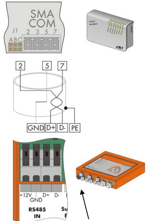
9. Connect the cable to the SOLTRK as shown in the figure above. Use the conductor colours you noted earlier.
