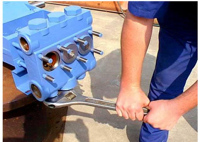
4. Remove the three valve covers (49), the threaded version is shown, or remove the six valve cover nuts (53) holding the valve cover clamps (51) and then remove the three valve covers (49) from the fluid cylinder. NOTE: Pumps that have threaded valve covers do not require removal of nuts and clamps.
