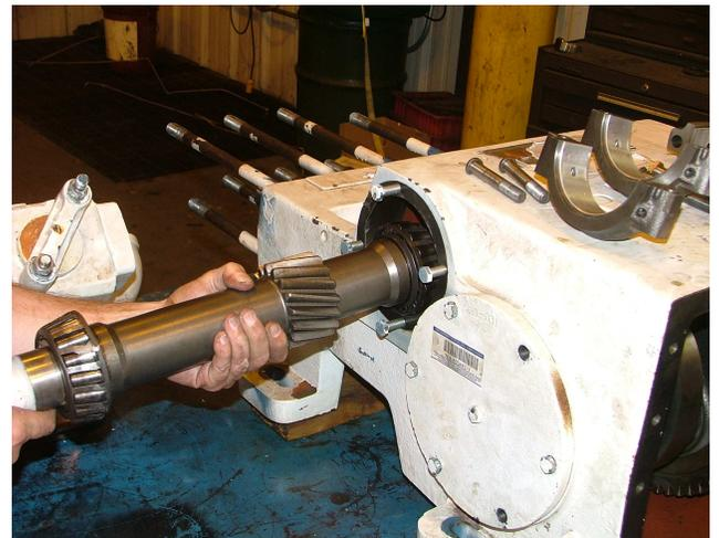
9. The pinion shaft (3) with bearings may then be removed from the drive side by using a brass rod (or other soft material) and mallet to drive the shaft out. The L16 pump will allow removal without the use of a mallet.
