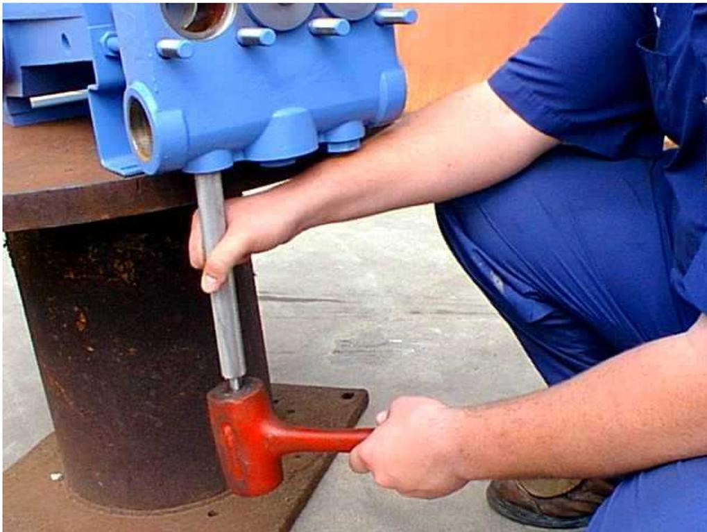
Picture 1: Removing the valve from the seat
