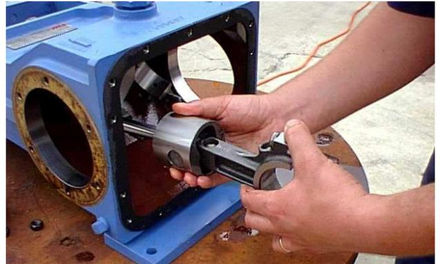
17. Remove the set screw (27) and slide the wrist pin (6) out of the crosshead (7) if crosshead or connecting rod (4) requires service. Keep components matched together.
