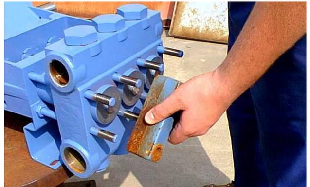
4. To access the piston cup seals (40), the cylinder cover clamps (57) must be removed (except as noted for L0918 in service tips above and some L06 models). Remove six of the nuts (61) holding the cylinder cover clamps (57) in place, and then remove the cylinder covers (54). Do not remove the two nuts (61) on the opposite corners of the fluid cylinder, as they keep the cylinders (39) and fluid cylinder mounted on the pump during this operation.
