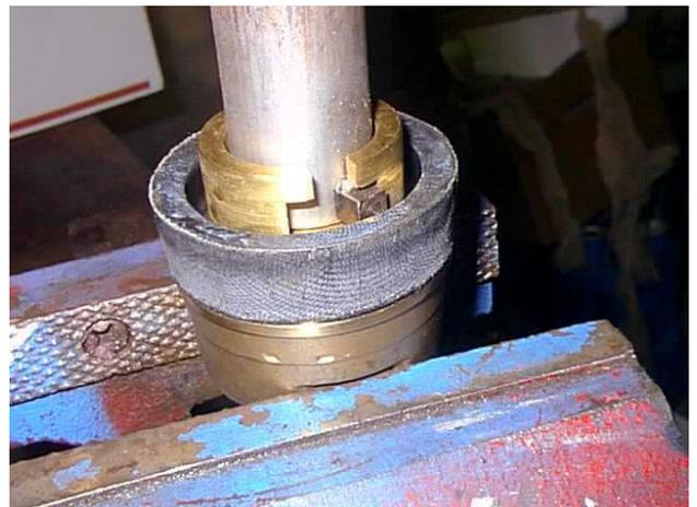
10. Inspect all parts for damage or unusual wear. Insure that the interior surface of the cylinder (39) is smooth and free of cracks or grooves. New piston cups (40) will fail prematurely if installed in liners with damaged bores. FMC strongly recommends that all three piston cups be replaced, not just those that show signs of leakage, whenever this type of service is performed. This will maximize operational time between service intervals.
