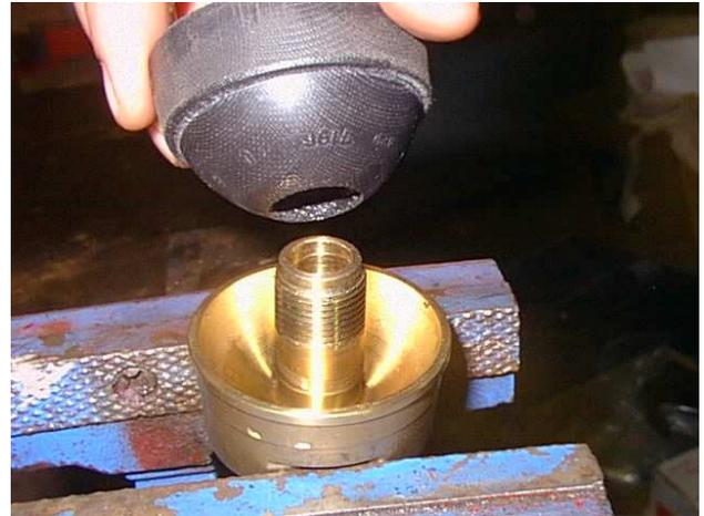
11. Reverse steps 3 through 10 to rebuild the pump after worn or damaged components have been replaced. FMC recommends that all seals and gaskets that are disturbed during the service procedures be replaced. This includes the rod seal o-ring (45) that is located on the piston/crosshead rod (shown) directly behind the piston assembly. Some pump models have the o-ring in a groove in the piston holder instead of a separate seal holder. Lubricate the piston cups and piston rods during assembly.
