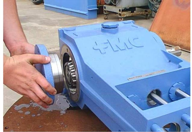
13. To remove the crankshaft (2) on pump models with no pinion shaft (some HD and HV), carefully move it through one side of the bearing housing opening in the power frame (1). The throws may have to be rotated as the crank is removed to clear the connecting rods. The crankshaft should be handled carefully to prevent the critical bearing surfaces from being scratched or damaged.
