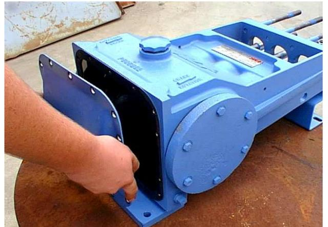
3. Remove all rear cover cap screws (29). Remove the back cover (15) and back cover gasket (16) from the power frame.
