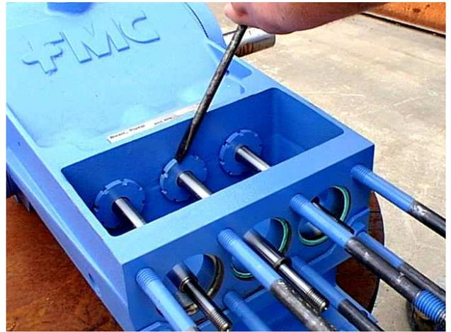
3. For L09 through L16 models, pull the seal holder (8) out of the pump frame and slide off of the rod. It may be necessary to insert a screwdriver or pointed tool into one of the holes in the seal holder on the L09 to help extract it from the power frame. For L11 through L16, it will require using two screwdrivers to slide the seal holder out of the recess. A slight rocking motion on the seal holder may aid in removal.
