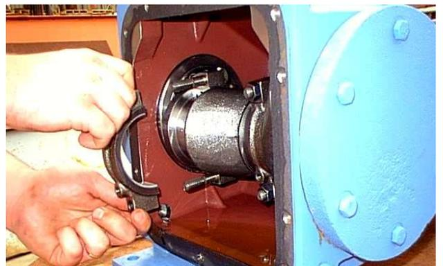
6. NOTE: Connecting rods and caps are matched sets and must always be reassembled with their original mate and in the same orientation. Note the numbered codes stamped on each half of the connecting rod assemblies and make certain they are installed as matched set and in the same orientation when re-assembling the pump.
