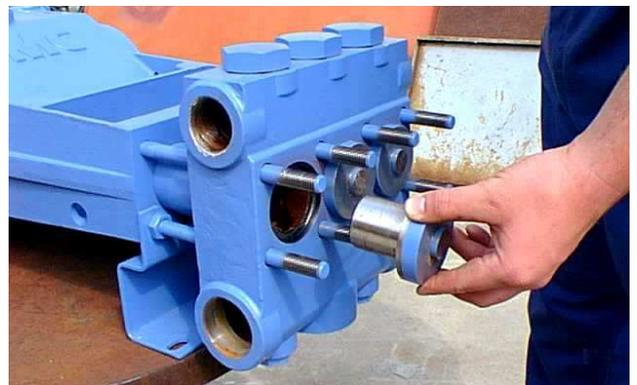
5. Some pumps may be equipped with a single cover plate that secures all three cylinder covers. For these models, all eight nuts (61) must be removed to facilitate removal of the cylinder covers (54). For some L06 models with no cylinder covers, the fluid cylinder (37) must be removed to access the pistons.
