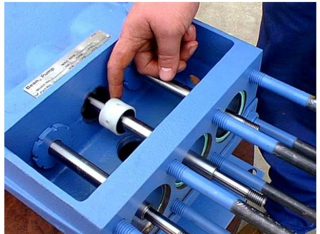
4. Remove the seal retainer gasket (11) from the power frame. Inspect the seals (9) and note the orientation of the seals prior to removal. The seals may now be removed from the seal holder and discarded.
