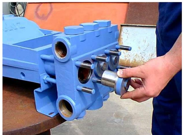
6. For AR valves refer to section 10.3.1. This document describes the methods for removing and installing the AR valves.
