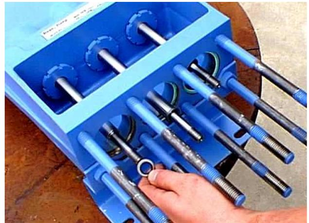
12. Tighten all fasteners to the values specified in Fastener Torque Requirements, Section 11.0 of this manual.
