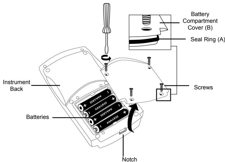
To ensure that the instrument is waterproof:
