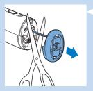
5 Remove the bottom part of the handle and cut the two wires that connect the bottom part to the appliance.
