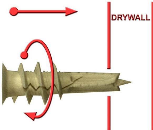
4. Insert the screw into the anchor and use the screw driver to tighten it into the anchor.
