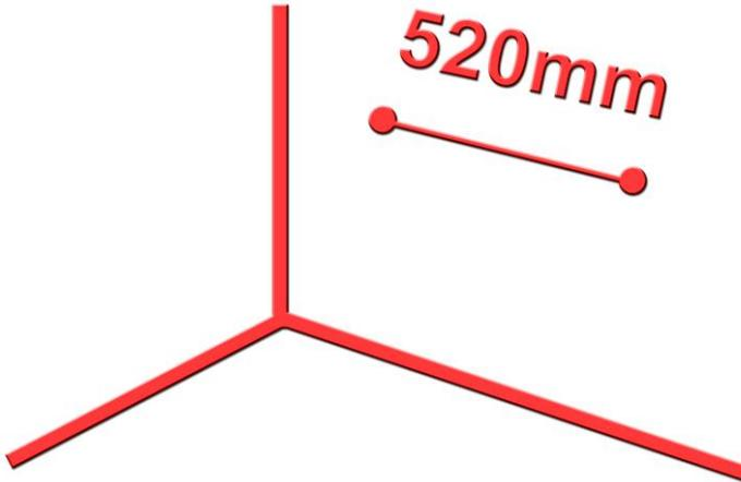
To mount the Sound Bar you need to have 520 mm of horizontal space on the wall.
