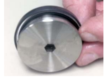
Figure 8: Replacement piston seal (Spring faces up)
