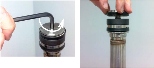
Figure 7: Separate retainer from piston
