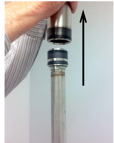
Figure 5: Remove pump cylinder
