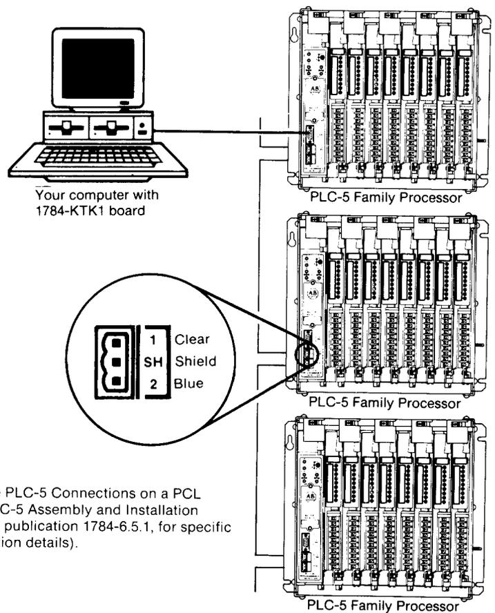
Multiple PLC-5 Connections on a PCL
