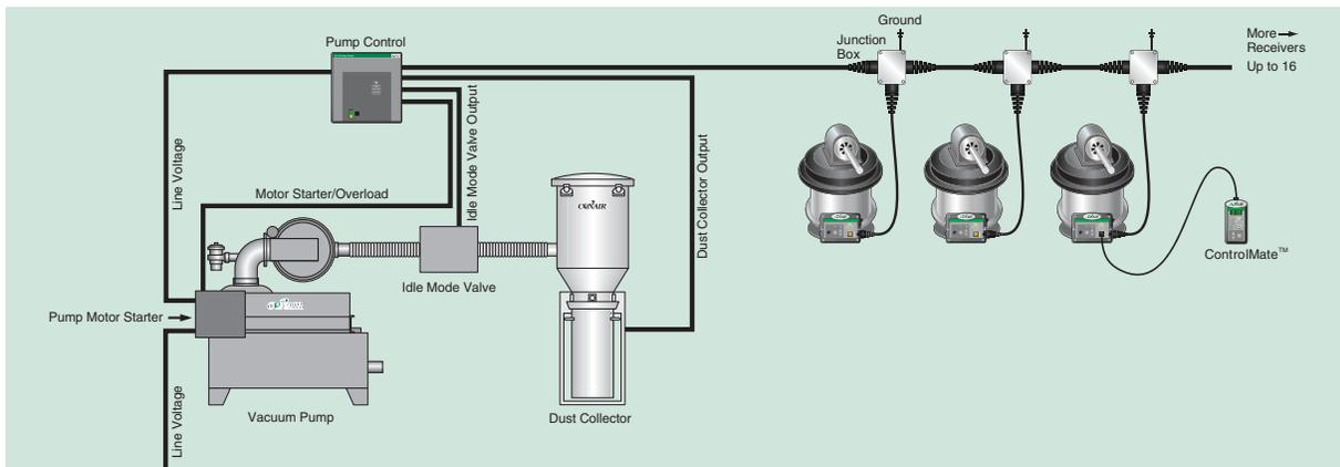
A signal from the receiver's demand switch indicates to the individually mounted ELC-16 on the receiver that it requires material to be conveyed to satisfy its demand. The ELC-16 then communicates its need for material to the pump control via a CAN open network. The demand signal from the ELC-16 is then added to the pump control's queue. The vacuum pump control will then permit the receiver to load on a First-In/First-Out (FIFO) basis.
