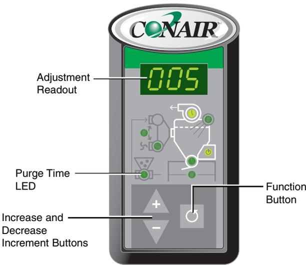
**NOTE:** When using purge, the ratio layer settings will default to one (1). (One layer of virgin material and one layer of regrind material regardless of the ratio percentage setting.)
