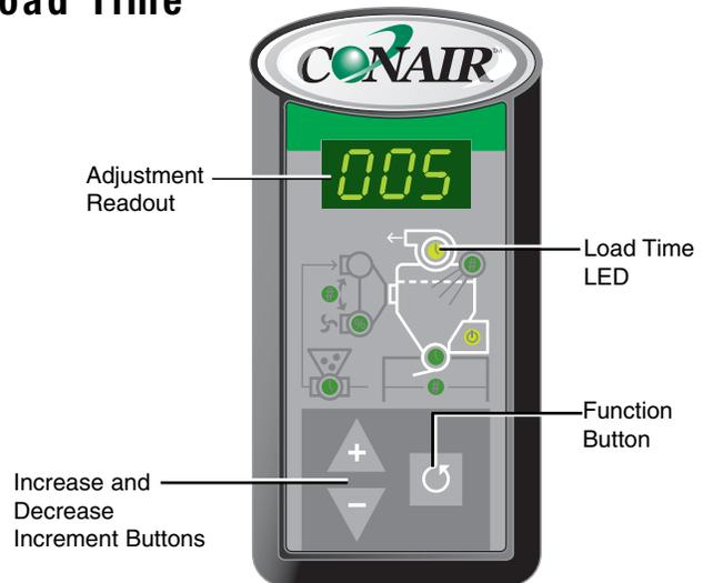
Setup for Load Time using the optional ControlMate pendant will operate exactly as the ELC control. *See Operation section entitled, ELC Loading Control Operation, Load Time Adjustment.*
