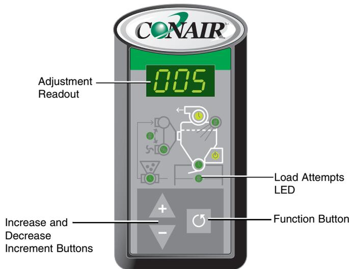
On initial start-up and fill-up of your vessel, the Load Attempts setting will be ignored. Only after the initial fill-up will the Load Attempts setting be used by the control. However, if you are using the loader/receiver to convey regrind from a granulator, setting the Load Attempts to “0” will allow unlimited load attempts to avoid nuisance alarms.
