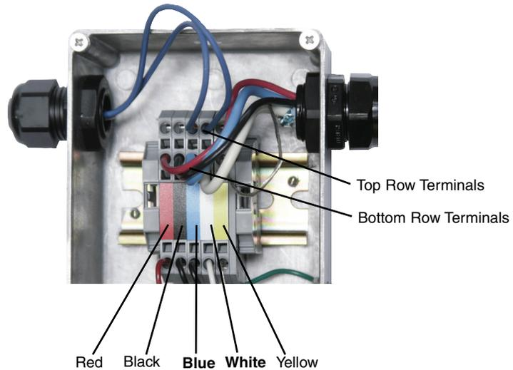
(Left-side termination resistor connection)
