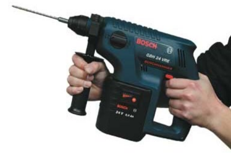
Figure 3-1. Example of drill with auxiliary handle (on the front of the drill)
