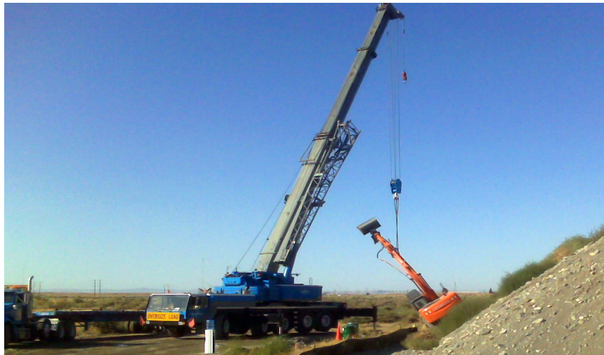
Figure 1-2. Mobile crane lifting trackhoe upright
