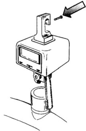
3. With the sling in place, press the "ZERO" button to set the system zero. The digit "0" will pan across the display for a few seconds then the display will read "0,0".
