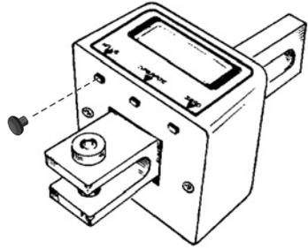
1. Attach the top hook of the SR 801 Scale to the boom or the lifting strap of the patient lifter. Make sure that the hook is fully engaged, and the safety screw is properly installed.
