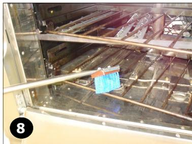
9. Use long handled scraper supplied, to scrape off any burnt-on product from oven internal surfaces.
