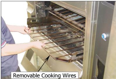
4. Check tray stop arms move freely and stop racks in unloading position when door is opened.
