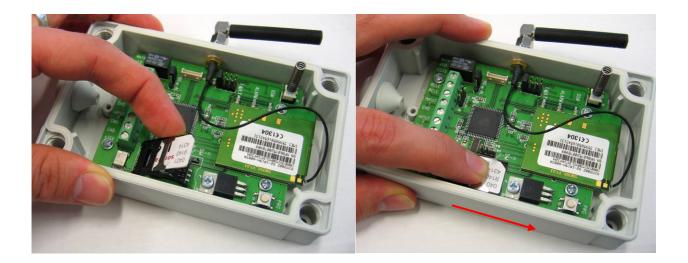
3. S Close the holder by lowering it down and gently pushing the metal clamp until it locks into position.
