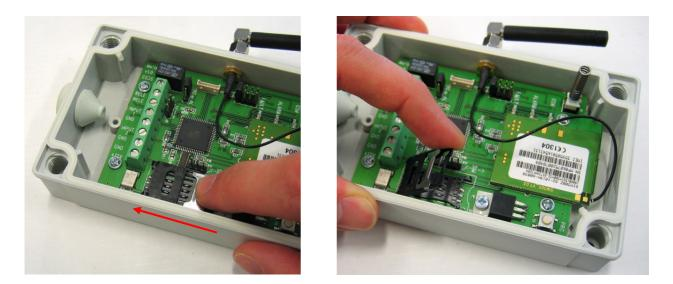
2. Place the SIM-card as presented in the picture. Close the holder by lowering it down and gently pushing the metal clamp. Make sure that the bevelled corner points outwards from the PCB.
