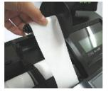
**ii.** Once the paper is attached, place the winding wheel into the holder in the back of the printer compartment. The portion the winding wheel with two disks should be situated on the right side. This will allow for contact with the winding motor and spinning of the wheel during operation.
