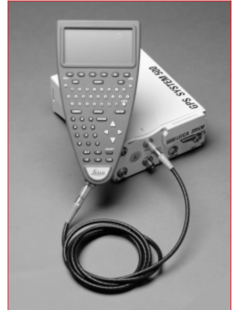
TR500 connected using the cable
