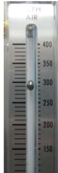
4. Adjust the flow meter adjustment knob so the flow is 300
