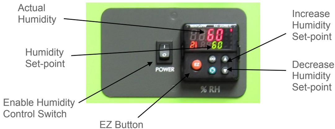
To set the humidity set-point, press the UP arrow to increase the humidity set-point by 1% RH. Press the DOWN arrow to decrease the humidity set-point by 1% RH. Pressing and holding either button will cause the set-point to scroll rapidly in either direction.
