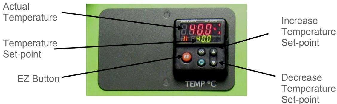
To set the temperature set-point, press the UP arrow to increase the temperature set-point by 0.1°C. Press the DOWN arrow to decrease the temperature set-point by 0.1°C. Pressing and holding either button will cause the set-point to scroll rapidly in either direction.
