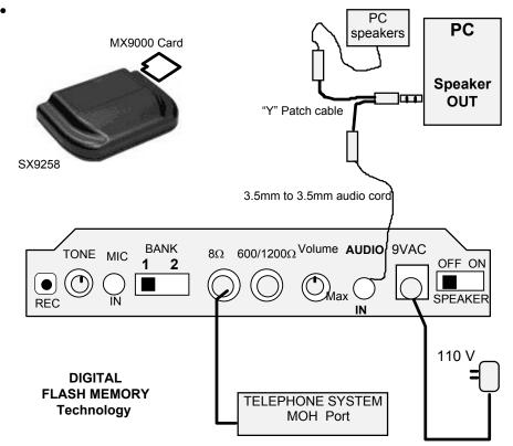
If the MX9000 card is already pre-recorded, audio playback starts automatically as soon as power is connected, the LED lights dance ON.
