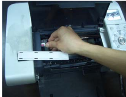
Adjust the tube length and move the cartridge carriage to the leftmost and rightmost. Make sure that there will be no block and collision when the cartridge moves.
