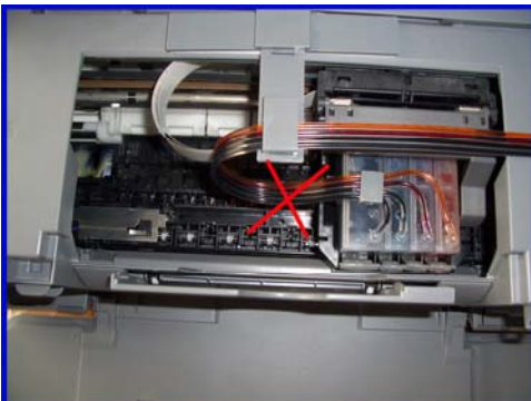
If the tube is excessive long, It is not ok.
