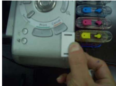
Take off the label on the shortest arm, and stick it on the right side of the printer. Then clip the tube through it.
