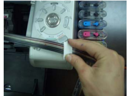
Take off the label on the shortest arm, and stick it on the right side of the printer. Then clip the tube through it.
