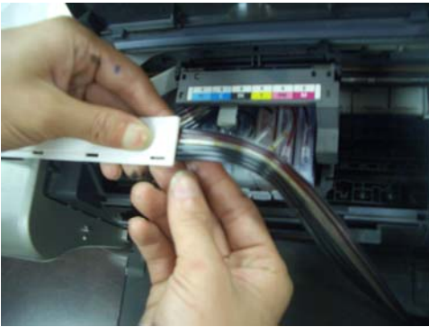
Clip the tube on the support arm.
