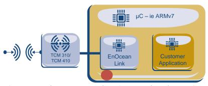
Figure 4. A Security implementation with EnOcean Link and an EnOcean gateway
