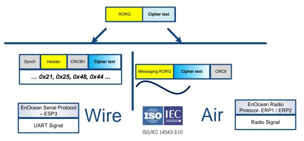
Figure 3 Seamless translation between serial and radio protocol
