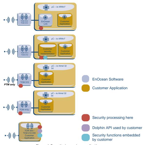
Figure 1 Security in receiver applications
