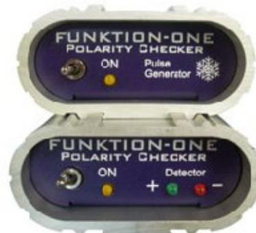
The ASPC1 is a two-part system comprising a pulse generator and a detector. The pulse generator allows you to inject a special test signal anywhere in the signal path whilst the detector microphone lets you check the resulting loudspeaker polarity acoustically. See the ASPC1 user guide for more information.
