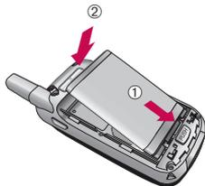
5. Press the battery until it clicks into place. Make sure that the battery is properly installed before switching the phone on.
