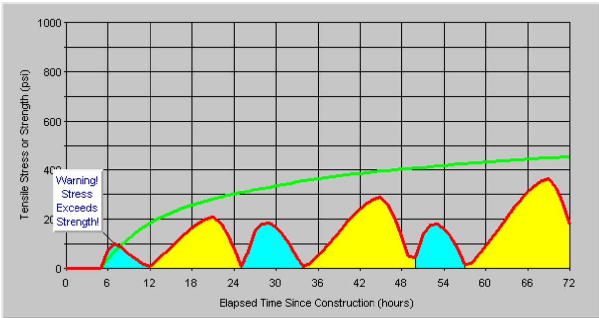
Figure 39. HIPERPAV output for case #2 - baseline with type III cement.
