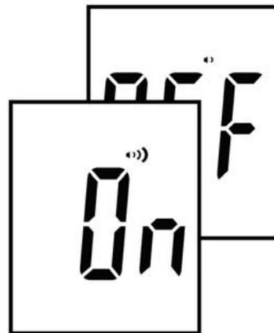
1. Insert batteries, the meter turns on automatically.
