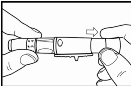
5. Pull on the sliding barrel of the lancing device until it clicks and then release.
