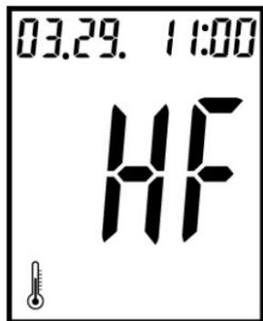
The "HF" and thermometer icon appears. Temperature is too high, outside the required range of 50°F-104°F (10°C -40°C). This alerts users that an incorrect result may occur if the test continues.
