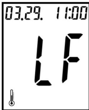
The "LF" and thermometer icon appears. Temperature is too low, outside the required range of 50°F-104°F (10°C-40°C). This alerts users that an incorrect result may occur if the test continues.
