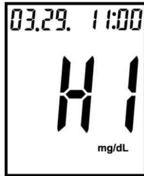
Test result is higher than 600 mg/dL.
