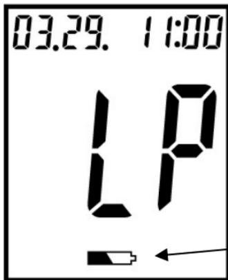
The meter uses two CR2032 Lithium Cell 3V batteries. Batteries will normally last for over 2000 tests. Other types of CR2032 Cell 3V batteries are also acceptable, yet the capacity of test times may differ. Install the batteries when you first use the meter or replace with new batteries when the "LP" (Low Power) message and the low battery symbol appear on the display.
