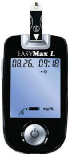
1. Put a test strip into the meter in the direction of the arrow. The meter will turn on automatically.
