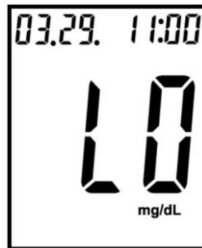
The test result is lower than 20 mg/dL.
