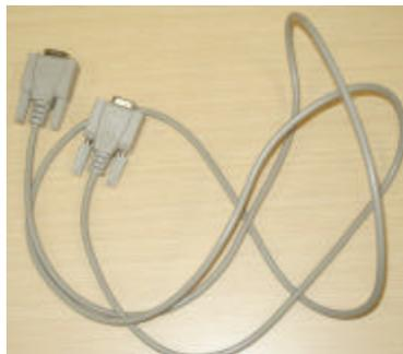
Figure 2 - DB-9 Pin cable
