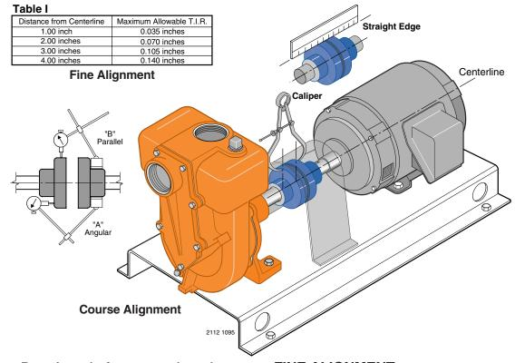
Rotating shaft can catch and trap clothing or body. Coupling guard must ALWAYS be in place when pump is running. Coupling guard shown in phantom for pictorial clarity.
