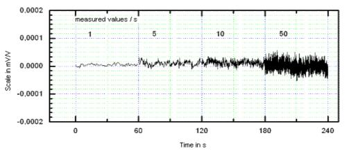
The best resolution at a datarate of 10Hz is at least 30000 digits, if you define the measured value compared to the amplitude of the maximum measured value (measured value maximum value tolerance).
