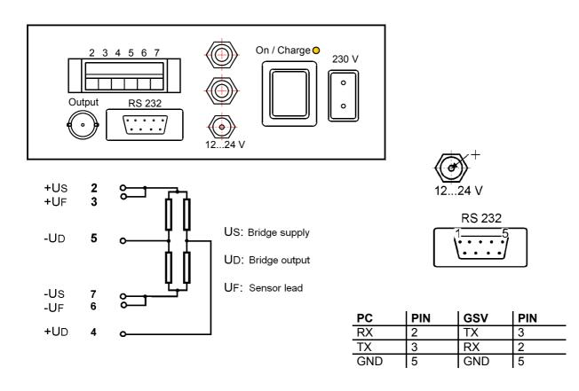
The connections 2 to 7 of the back plate are reffering to the connections of the connection panel.
