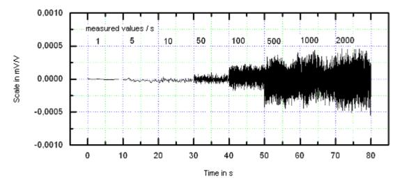
Resolution in the measuring range "2 mV/V" (2,5V supply voltage, JP1 in position 2)
