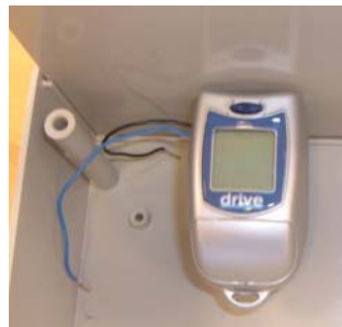
Figure 32. Pulse Oximeter Mounted Inside the Monitor
