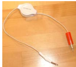
Figure 29. Thermocouple Probe on Retractable Cable
