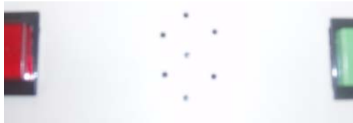
Figure 36. The Speaker is Mounted Inside the Front of the Monitor, Behind the Speaker Holes in between the Two Buttons
