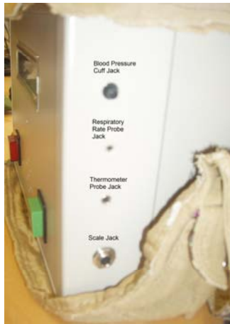
Figure 25. Side View of the Accessible Home Vital Signs Monitoring System Monitor
